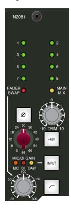
The Input Module hosts the Channel Input Selector, Gain and Trim, Phase, 48V, and High Pass Filter. All buttons are recallable using the consoles scenes.
