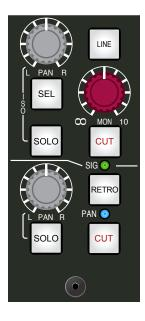
The Monitor path section features a rotary trim control and two selectable inputs, DAW and Line. Line, Retro, Cut, Solo and Solo Isolate are recallable.
