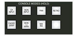
Depending on the application at hand, say for example recording as opposed to mixdown, the **Console Modes** section will change the global state of the console to reflect the most appropriate setup.
