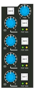
Each module contains two stereo (A & B) and three mono (Aux 1, Aux 2, Aux 3) **Auxiliary Sends**. The order in which Auxiliaries 1 to 3 are accessed is bottom to top respectively. A & B are situated above the three mono sends. All features other than the level controls in the Auxiliary Section are recallable.
